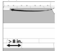
Step 3: Use left over plank at least 8" long to start next row. Tiles should by staggered 12" apart.
