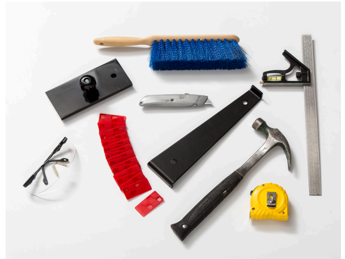
Tape measure, utility knife or saw, tapping block, pull bar, 3/8" spacers, T-square, safety glasses, broom or vacuum.
