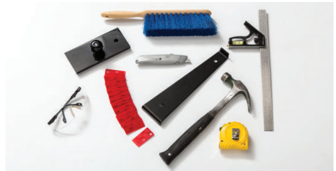
Tape measure, utility knife or saw, tapping block, pull bar, 3/8" spacers, T-square, safety glasses, broom or vacuum.
